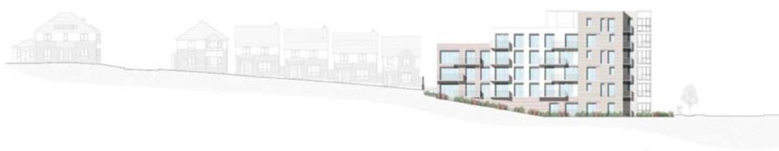
Fig. 8: Site section viewed from the south east showing the apartment building in relation to slope and adjacent houses. (CCK Architects)
